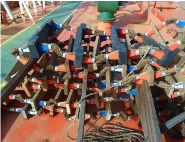
Figure 4. The pilot ladder that was used for the embarkation of the Security Guards.
